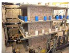
Researchers built an entire three-story building inside Purdue's Robert L. and Terry L. Bowen Laboratory for Large-Scale Civil Engineering Research to test the effectiveness of a simple, inexpensive method to strengthen buildings and reduce their vulnerability to earthquakes
