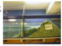
optimization of the typology of slope marine docks in order to lessen their main damage, the extraction of pieces from the external layer (loss...
